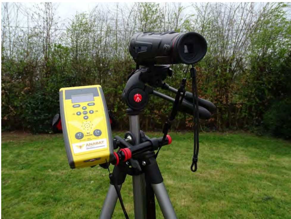
Thermal imagery scope set-up with tripod and full spectrum bat detector, being used by Tina Aughney in the BLE Monitoring.
