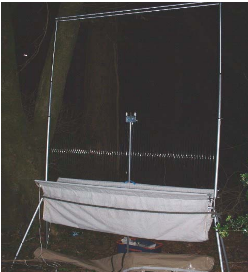
Plate 4: Harp-trap with Autobat sonic lure
