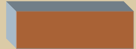
This 3D shape is 12mm high/wide and 50mm long, illustrating the dimensions of a suitable crevice for a single bat to use as a roost or access a roost.
