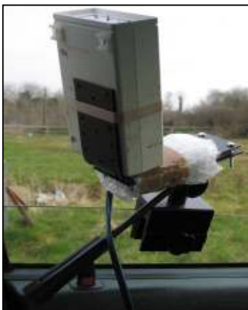
A bat detector clamped to a car passenger window. The lead links the bat detector to a minidisc recorder.
